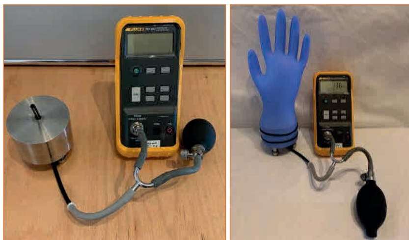
Fig. 3: Pressure measurement over 30 minutes at approximately 15 mbar.
